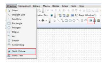
After the static picture component is selected, drag by the left key of the mouse, and then the corresponding properties window will pop up.
